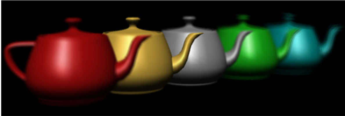
Figure 1: Depth of field effect using frustum jittering. Note the gold teapot is the focused object.
