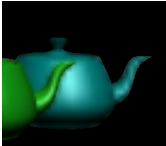
Figure 7: Artifacts from Reverse-mapped DOF. Note the texture artifacts from magnification in the cyan teapot. And that the outline of the teapot remains sharp through it is at the far extreme of the DOF blurring. Also note that the green teapot 'bleeds'.
