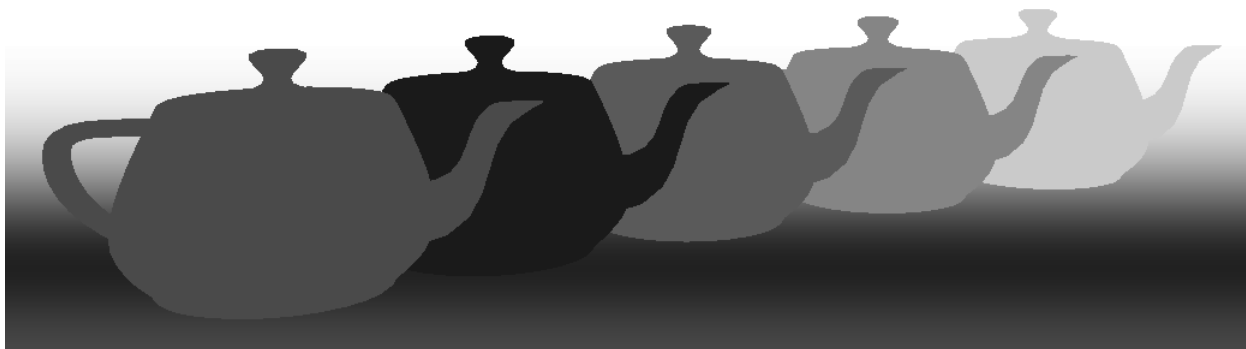
Figure 4: The Z-depth of the scene as rendered to a texture.
